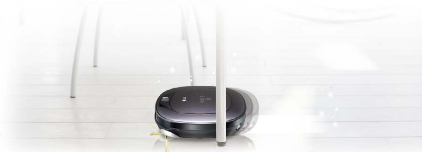
Ultrasonic sensor of HOM-BOT SQUARE senses wider and more precisely. It can even sense glass and transparent objects.
